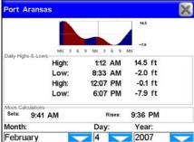
The Port Aransas, Texas tide symbol in the left figure has been highlighted with the cursor. In the right figure the Information button has been selected to view tidal information for that station.
